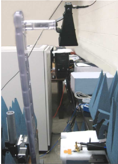
Fig. 8. Photo of the reconfigurable antenna measurement system (RecAMP) during the pattern measurement of the reconfigurable antenna.
